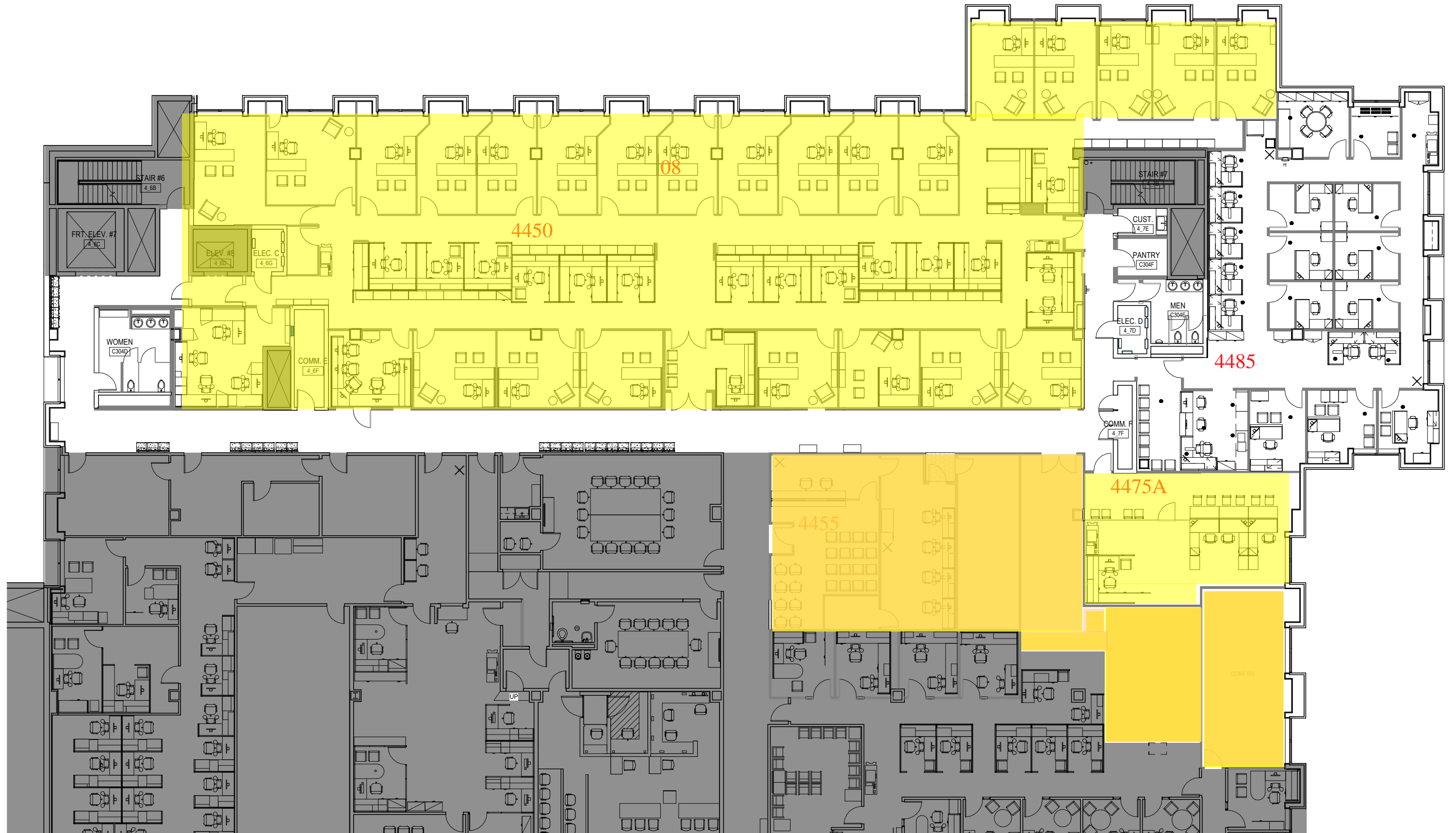
Figure 4 - Locations with ACM Joint Compound (Yellow highlight)
