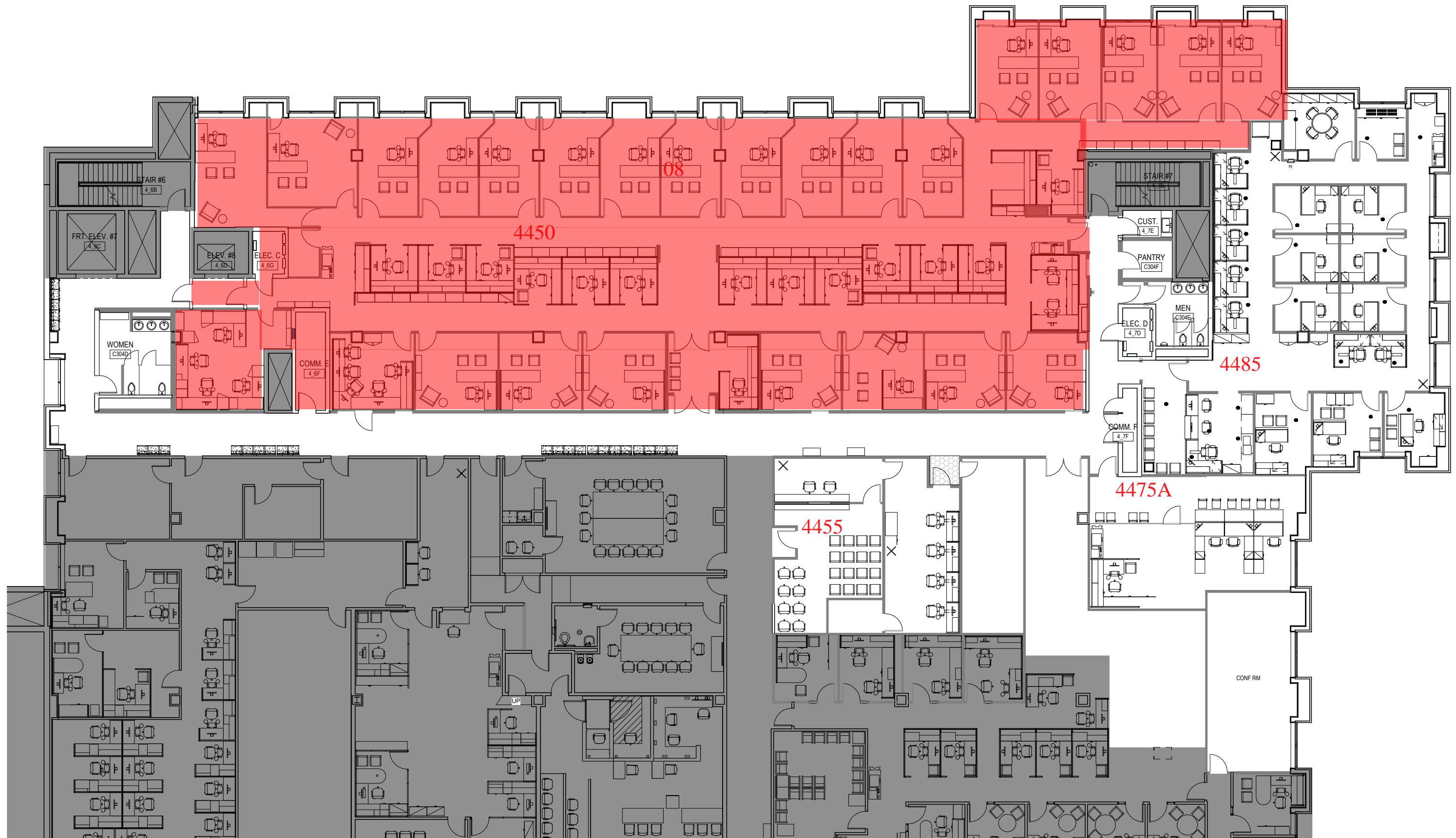
Figure 2 - Locations with ACM Floor Tile (Red highlight)
